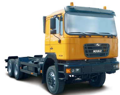
KRAZ H23.2M chassis with MAN cabin
