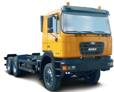
KRAZ H23.2M chassis with MAN cabin
